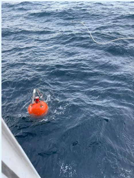
Recovery of an ADCP buoy. Copyright Knút Olsen.
